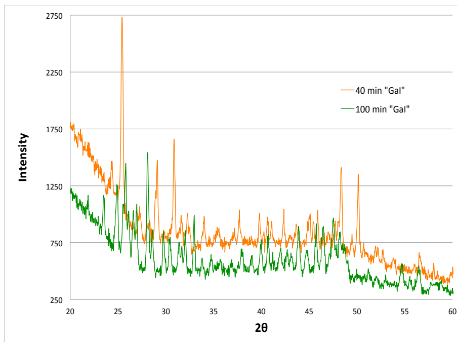
Figure 2: Top: Powder diffraction patterns of “Gal” as a function of reaction time 40 minutes (orange), and 100 minutes (green). The uneven baseline is a result of the scotch tape used to prevent exposure of the sample to air.
